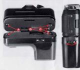
1 Hold the back of camera at a right angle to the winder as illustrated, matching up each of the terminals (a) (a) and (b) on both the winder and the camera with your eye.
